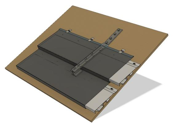
7, If a log type snow fence is desired, plan the snow fence holder brackets to be installed just above bearing walls to carry the extra weight. After installing the Panels below the planned snow fence, install the snow fence brackets as shown above. There is no need to cut the Panel's back hem, just bend the hem up a little to accommodate the bracket's thickness. Fasten the snow fence brackets with appropriate fasteners.
