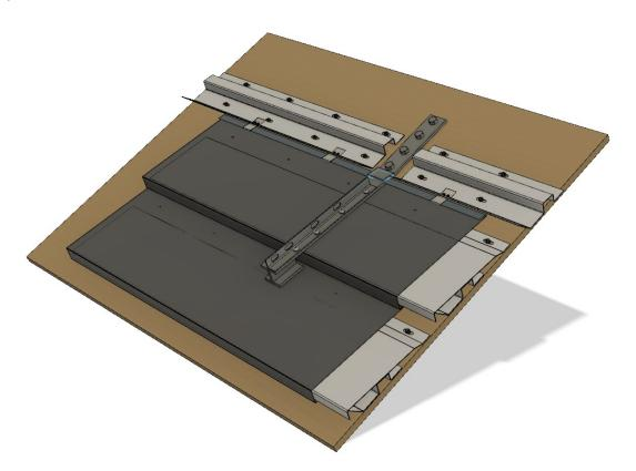
8, Install the next row sub-support, keep a 1 inch gap between the snow fence holder bracket and the lower sub-support profiles.
