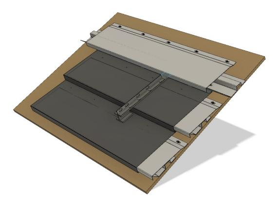
9, Install the next row's upper sub-support profile, it will need to be notched out a small area where it would otherwise interfere with the snow fence holder bracket.
