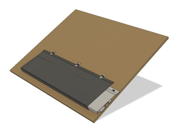
4, Install the first roofing Panel as shown above by interlocking its lower edge into the drip edge and fasten the upper edge, by aligning with the line or chalk line, using the supplied stainless steel clips.
