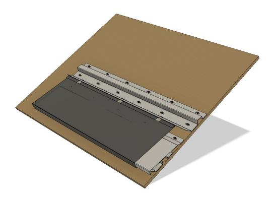
5, Install the lower sub-support profile for the next row of Panels, appropriately aligning it with the first installed Panel.
