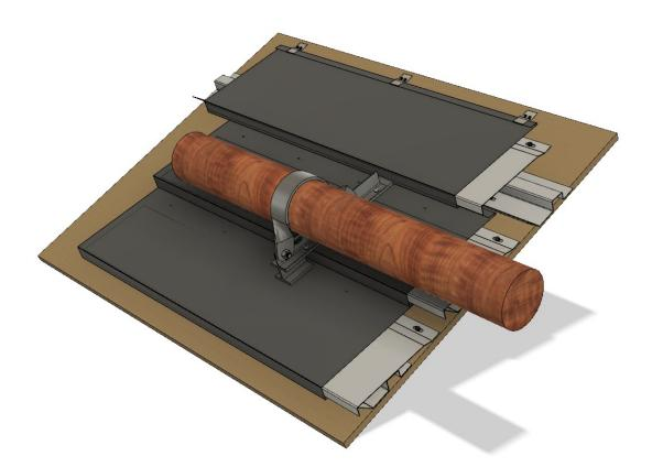
12, Fasten the log with the supplied log-fastener clamp onto the bracket. We recommend using no longer than 12 feet long logs as snow fence, using 2 sets of snow fence brackets per log, each bracket installed 2 feet from the ends of the log for best use of snow holding power.
