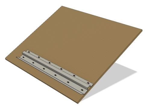
2, Install the lower Panel sub-support profile, perfectly parallel with the drip edge and at the precise distance from the drip edge metal.
