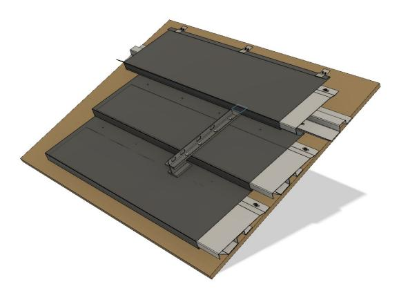
10, Install the next Panel. This panel too needs to be notched out a tad where the Panel would otherwise push against the snow fence bracket.
