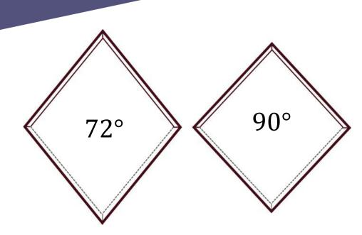
Our standard Diamond Shingles come in 4 different sizes and two degrees, 72° and 90°. That being said, we can make our diamond shingles in just about any size and shape, and can also have patterns pressed into them!
